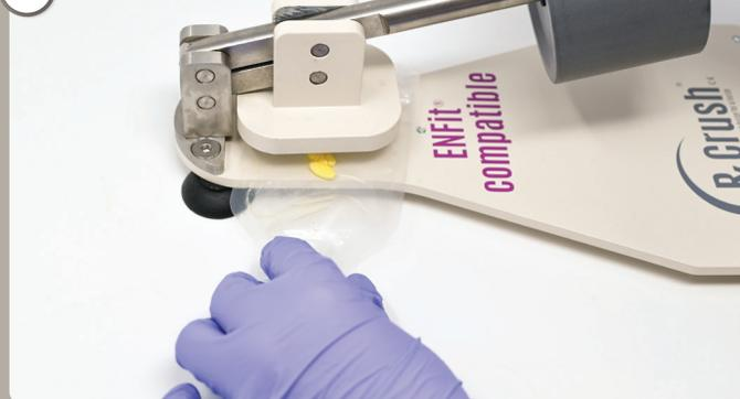
Hold syringe to the side and use the crush plate to crush pills by moving handle up and down.
